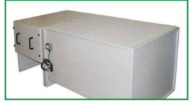
The Filter Bench works on the principle that any dust or fumes generated by the operator are quickly drawn down through the perforated worktop. The internal filters then clean the air, which can be either returned into the workplace or vented to atmosphere. These units are simple to operate and quick to install.
